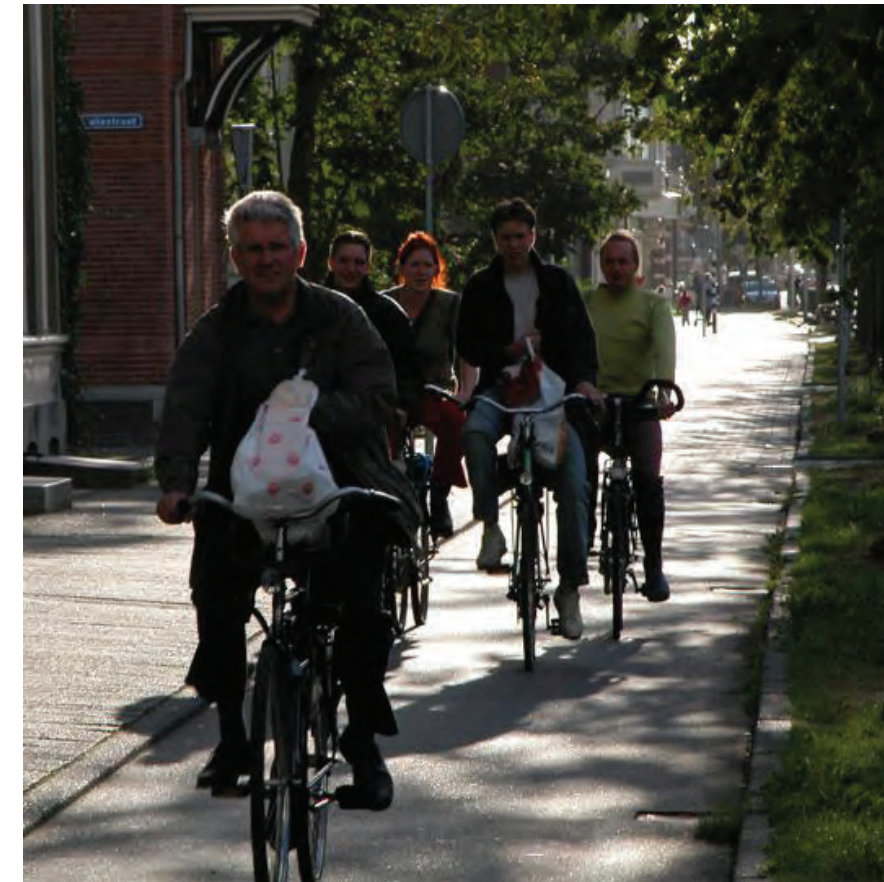
2+1 Width: Two-abreast cycling with room for overtaking
